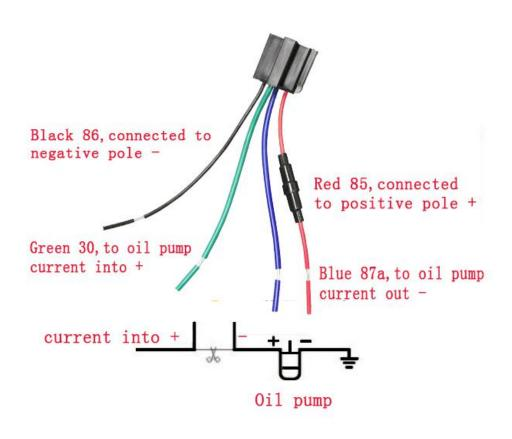
Remark: if you want to cut off the oil, it needs to connect external power, do not use the built-in battery.
